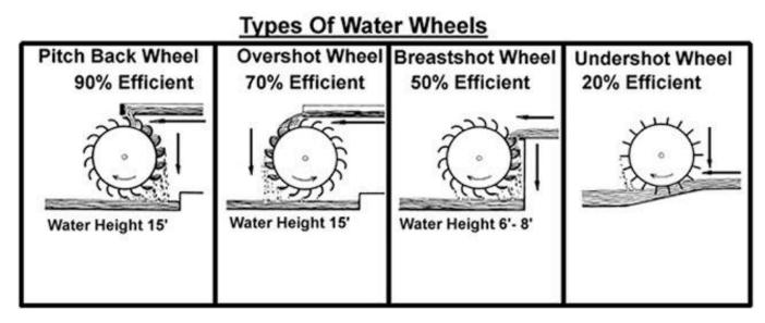
Medieval wheels would have been made of wood, but later they were replaced by cast iron, which was stronger and harder wearing. Along the Wandle most of the wheels were undershot or breastshot. There were some overshot in **Carshalton and Waddon Mills**; overshot wheels were proved to be the most efficient type.
